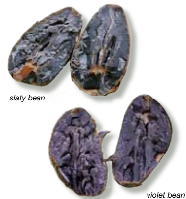
Cutting Test This is a visual inspection of cut beans. Color deviations are detectable which are indicative of fermentation problems or spoilage (moulds).
